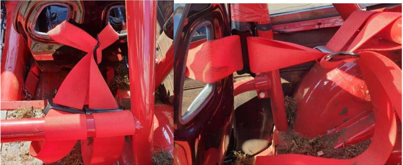
The sideview is taken with a Scrutineer pulling the belts tight, notice the slack caused by this extra buckle hitting the rear of the seat. Not only does this slack mean the driver is not properly restrained, but in an incident the loading of the belts would be passed directly into the seat back which could result in seat failure.
