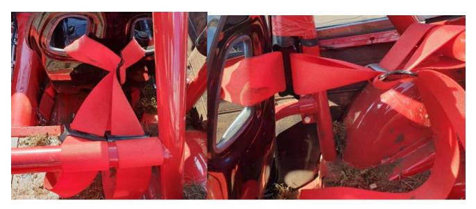
The sideview is taken with a Scrutineer pulling the belts tight, notice the slack caused by this extra buckle hitting the rear of the seat. Not only does this slack mean the driver is not properly restrained, but in an incident the loading of the belts would be passed directly into the seat back which could result in seat failure.
