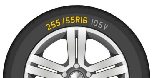
This string of numbers (in the image 255/55 R16) indicates the size of the tyre. This is important as you will need to ensure that any tyres you fit to your vehicle are the correct size as specified in your vehicle handbook. These tyre numbers mean:
